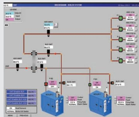
An upgrade to the building's DDC controls allowed for heating demand feedback from each system zone. The critical zones within the school are identified and the system flow and temperature are reset based on the building heating demand. This control strategy drives the supply and return water temperature as low as possible, increasing the condensing boiler efficiency.
